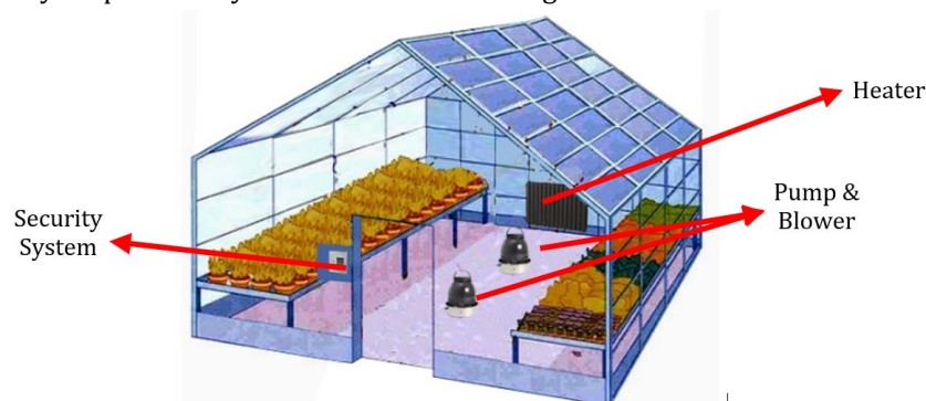
Figure 5. Design of hardware installation layout plan in green greenhouse
